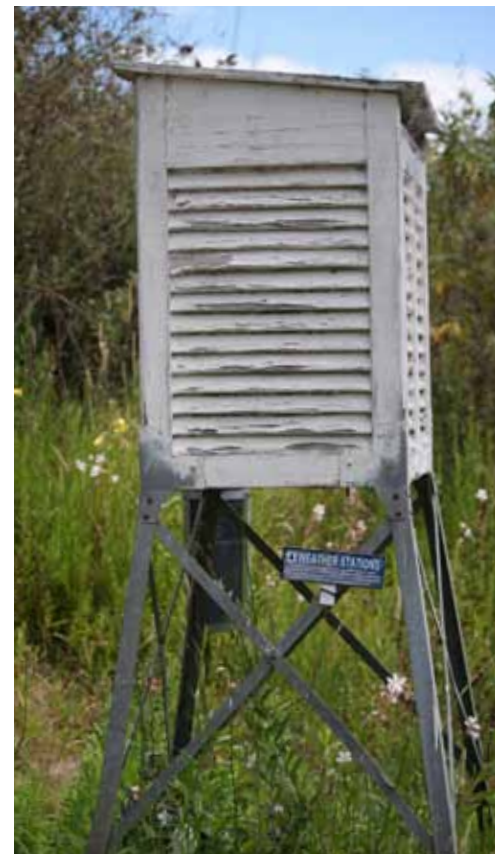
Weathered weather station where highs, lows, and rainfall has been recorded since 1930. Photo by J. Bennett.
